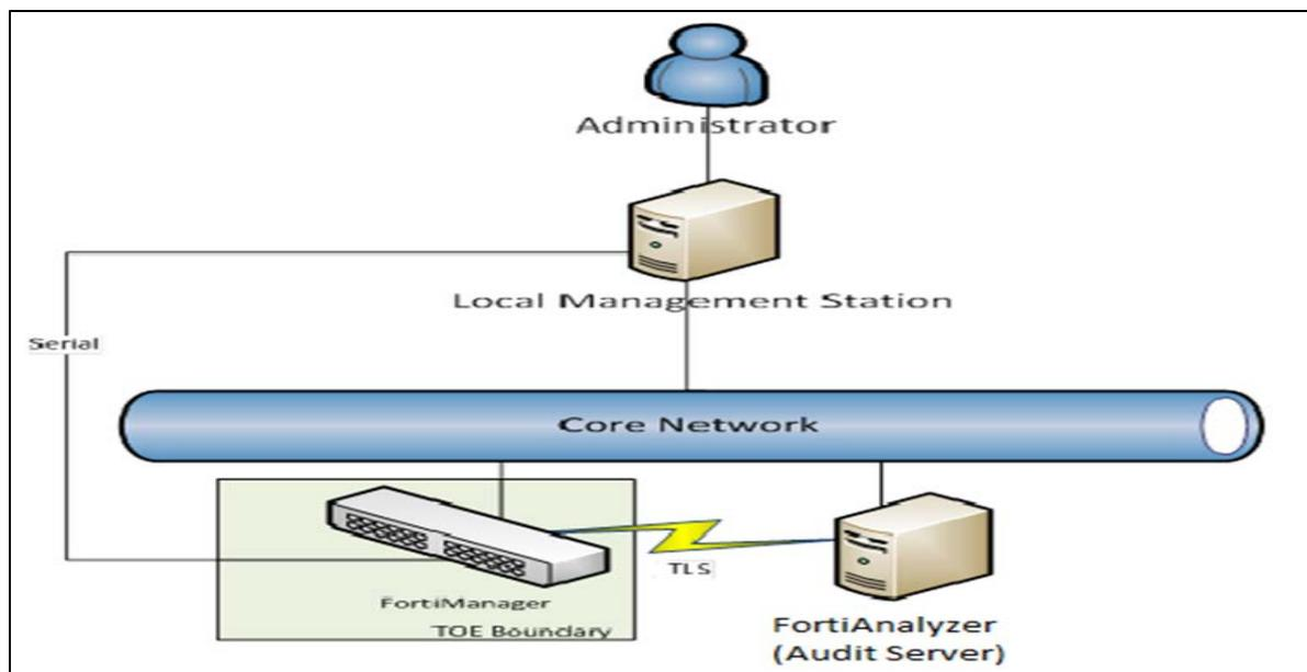
**Figure 1 TOE Architecture**
